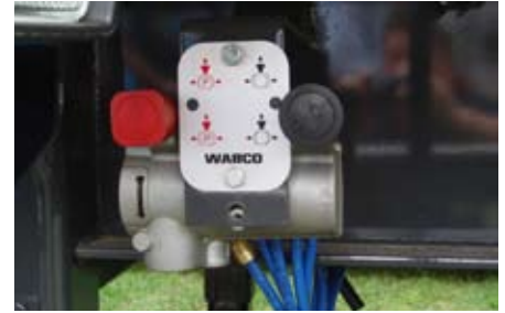
The Brussels valve is the red one. The instructions are clear and easy to understand.
