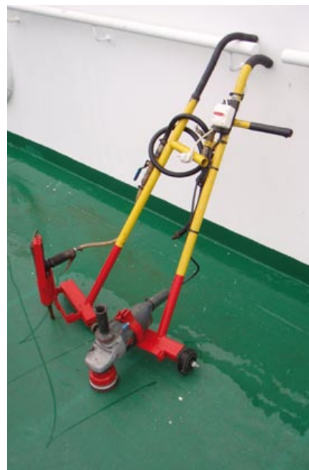
The trolleys reduce loads and vibrations from both needle guns and angle grinders.
