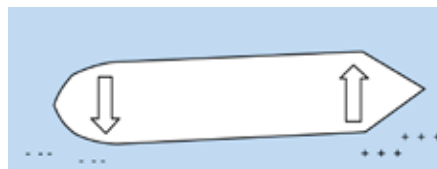
Illustration of the bank effect when sailing in a narrow passage. The plus signs indicate increased pressure and the minus signs indicate decreased pressure. The arrows show lateral forces acting on the ship.
